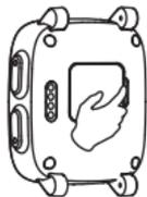
1. Power off the device and open the plastic SIM cover.
