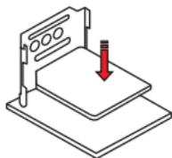
2. Push and flip open the metal SIM slot cover and install the SIM card with the metal pin facing down.
